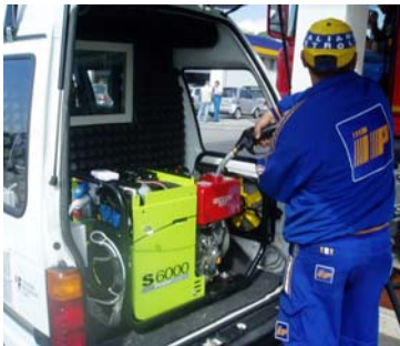
The Diesel Motor/Generator system.
