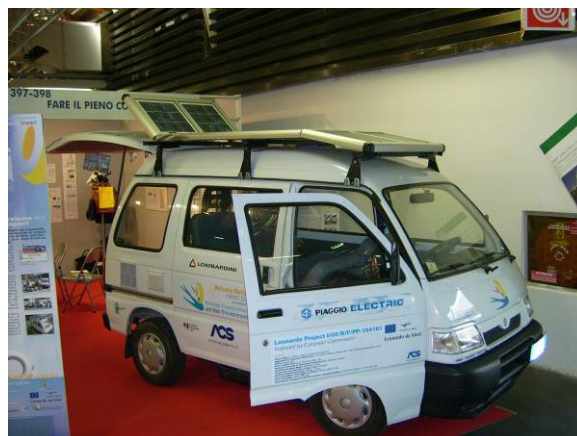
Fig. 2 – The prototype of Hybrid Solar Vehicle.
