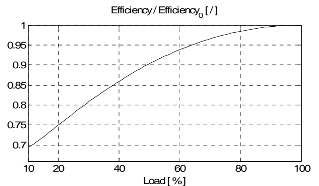
Fig. 5: Off-design operation - turbine efficiency
